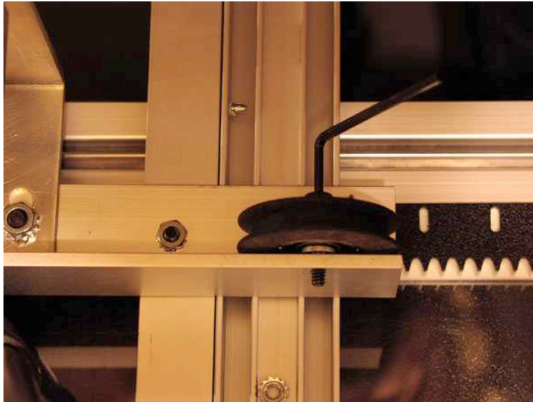
(29) I removed the shoulder bolt with the old wheel using an allen wrench.
