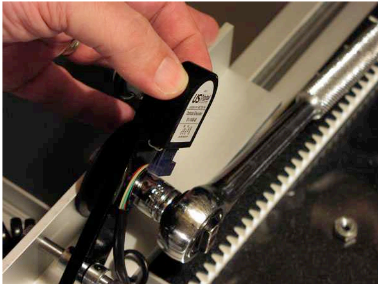
(15) Holding the S/R sensor out of the way, I removed the parking wheel.
